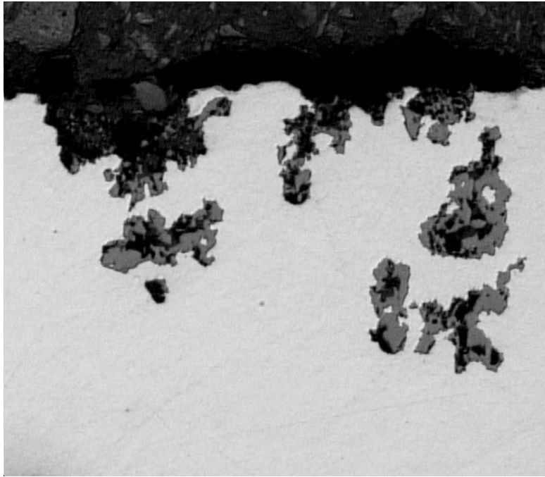
Figure 2 Typical cross-section of formicary corrosion, noting the penetration advancing parallel and perpendicular to the cut surface. (250X original magnification)
